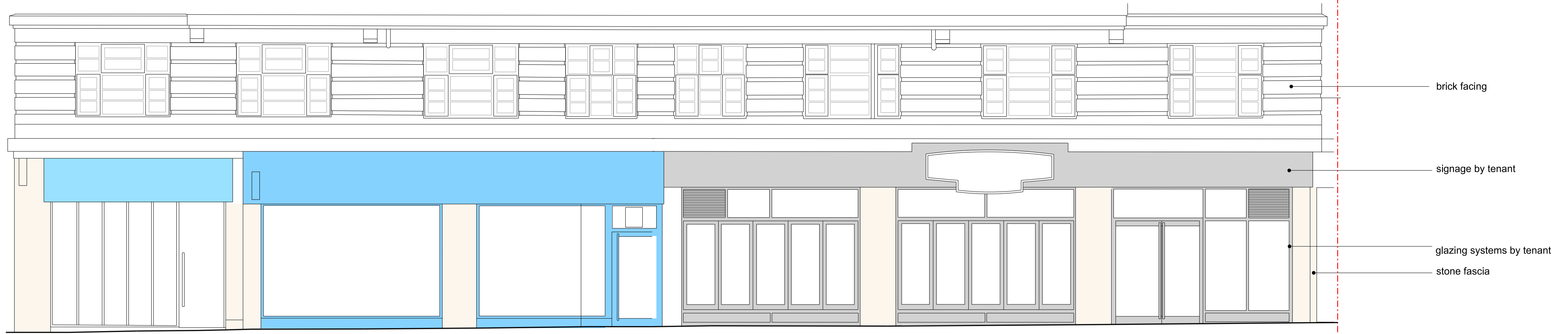
existing partial elevation 1
