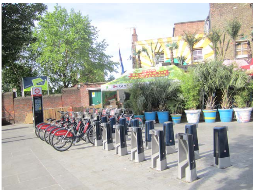
Figure 3.1: Double row docking station on footway
