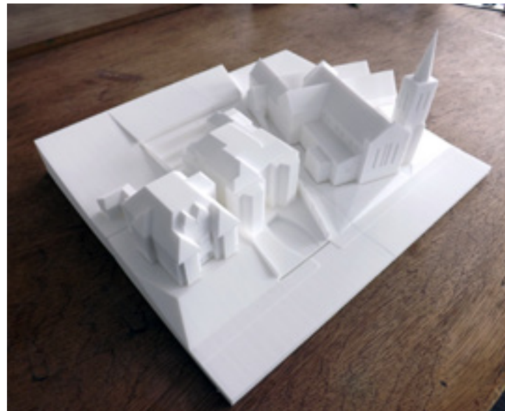
Model constructed in order to test the mass and volume of the proposal, respecting the neighbouring sites
