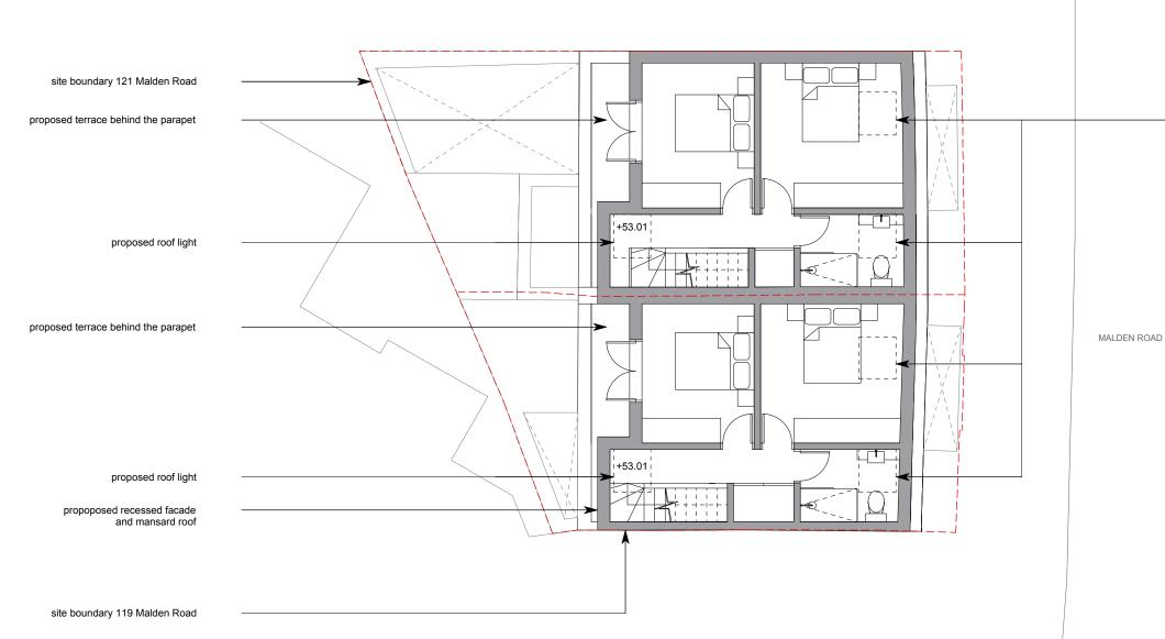
**Proposed Mansard Roof Floor Plan** scale 1:100@A3
