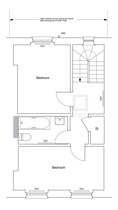
Existing, non fire-rated flush internal doors to be replaced with solid timber flush fire doors.
