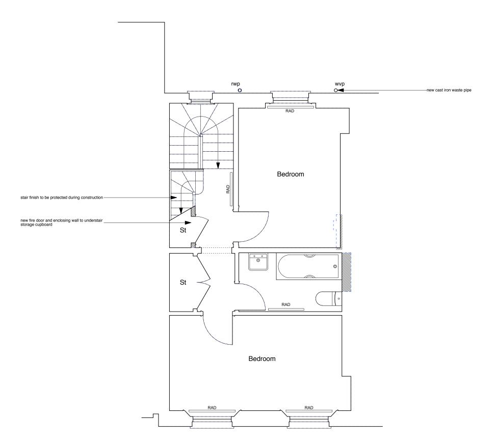
Existing, non fire-rated flush internal doors to be replaced with solid timber flush fire doors.
