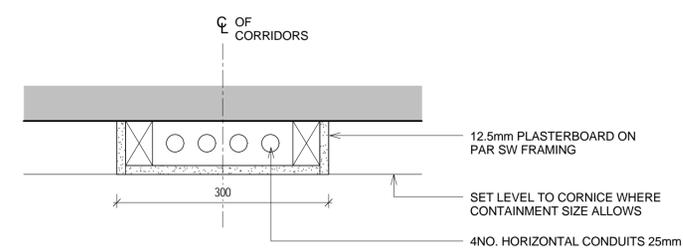
**3** CONDUIT DETAIL - SECTION A-A
