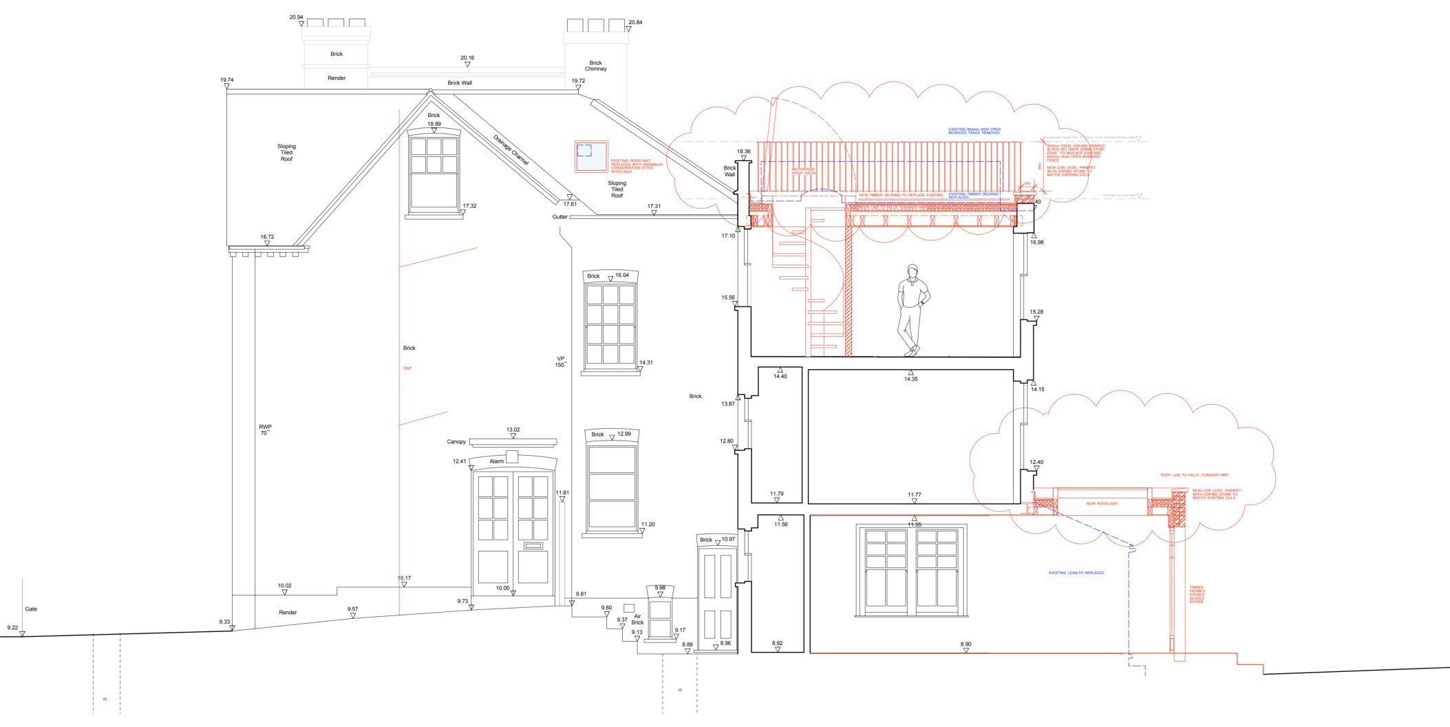
GENERALLY: EXISTING SINGLE GLAZED TIMBER SASH WINDOWS REPLACED WITH DOUBLE GLAZED TIMBER SASH WINDOWS PAINTED WHITE TO MATCH EXISTING
