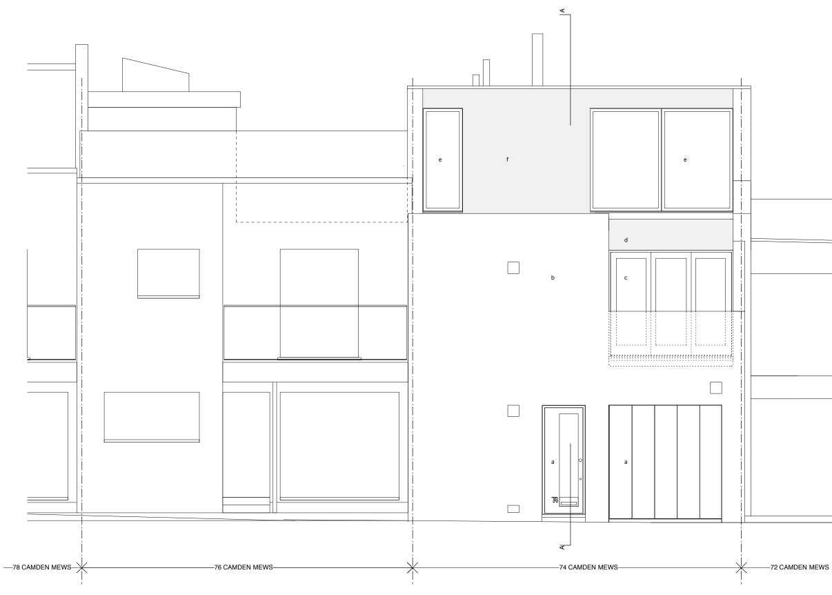
KEY a. existing doors b. existing brick c. existing windows d. new zinc fascia (to replace existing)
