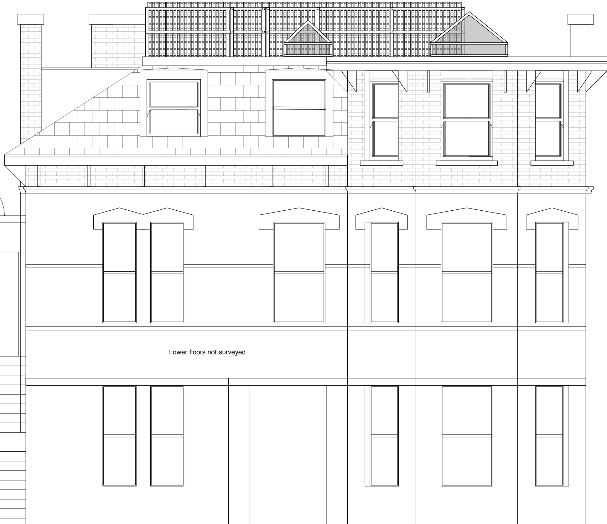
Existing railing - Key Clamp handrail, painted pink, with guarding panels of timber garden trellis
