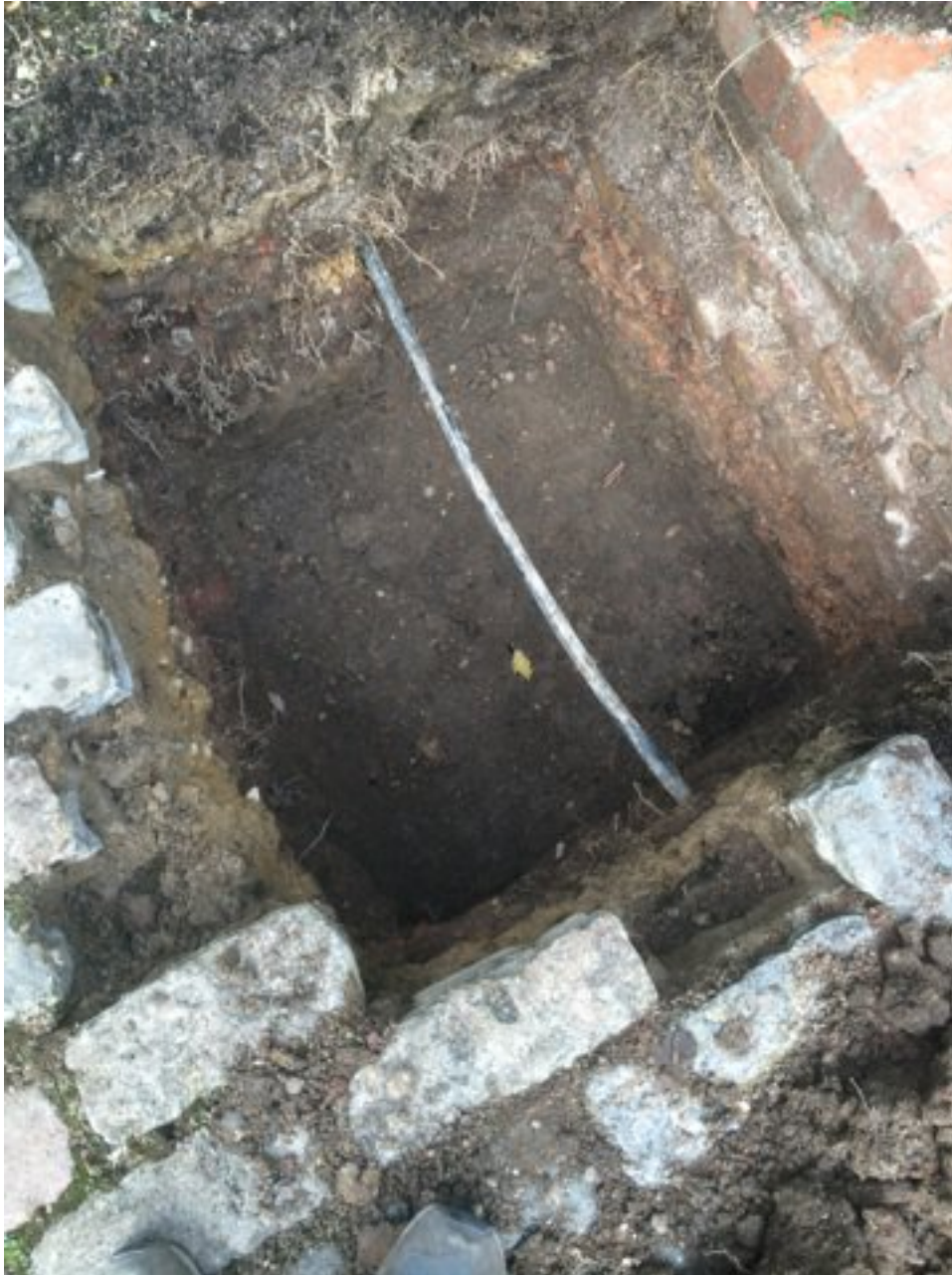
Photograph 2: Trial Pit 1 with fibrous roots only. Pit dug to 900mm depth and logged by Capstone.
