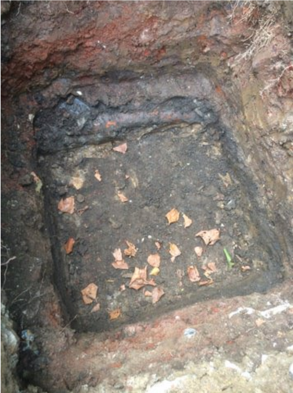
Photograph 3: Trial Pit 2 with fibrous roots only. Pit dug to 900mm depth and logged by Capstone.
