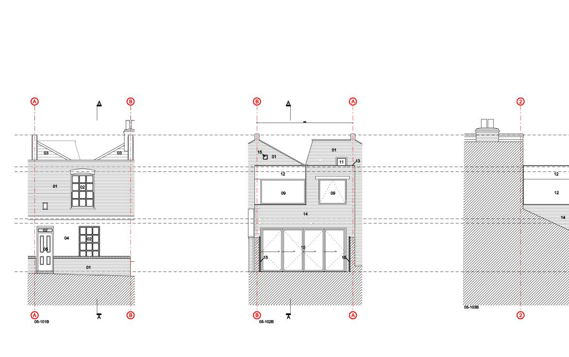
01 PROPOSED FRONT ELEVATION SCALE 1:100 AT A3
