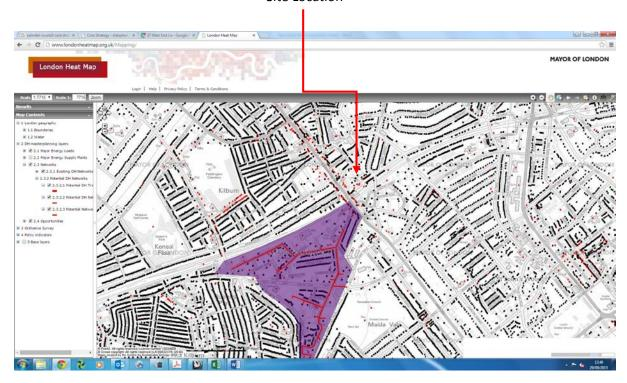
The study identified the area of the development on West End Lane with a potential District Heating network, however the costs involved in extending the potential DH network would outweigh the advantages achieved from such a connection due to the size of the development. This is demonstrated clearly from the London Heat Map (http://www.londonheatmap.org.uk) snapshot.
