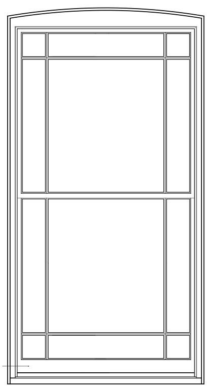
Solid timber sash frame, to receive white paint finish to match existing
