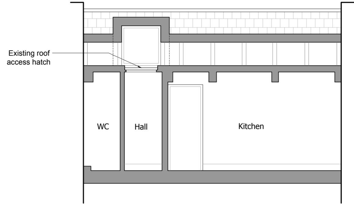
1 Internal elevation C as existing
