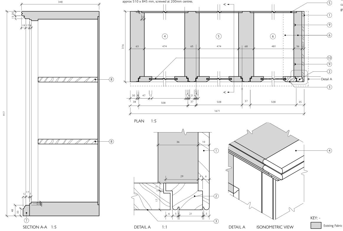
Take off existing cupboard door and take elements apart. Cut a (10)chamfer into the bottom edge of the panel and supply and install a new section of mahogany to extend panel, approx. 141 x 50 x 7mm. Cut in new mortise joints in existing stiles and piece in where old joints in existing stiles and piece in where old joint removed. Re-hang cupboard door.
