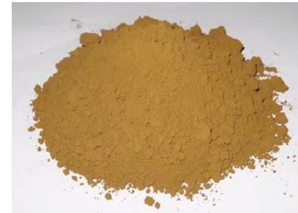
Figure 2-1 Titanium nitride powder is the base material used for the TiN PVD coating process
