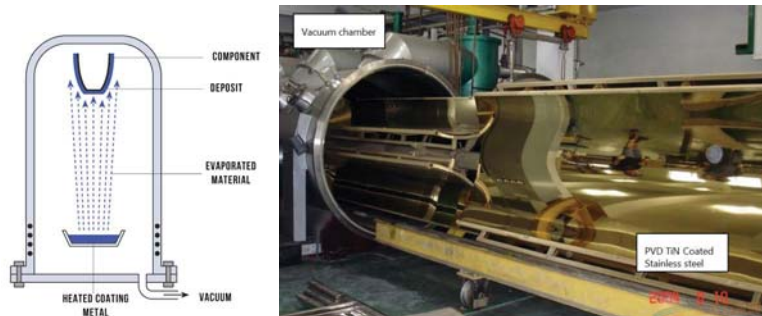
Figure 2-5 Schematic describing the sputter PVD process commonly used for decorative coating applications and Example of a PVD coating chamber with a TiN PVD coated stainless steel sheet (source: Cosmone.com, Dongguan Huicheng Vacuum Technology Co. China)
