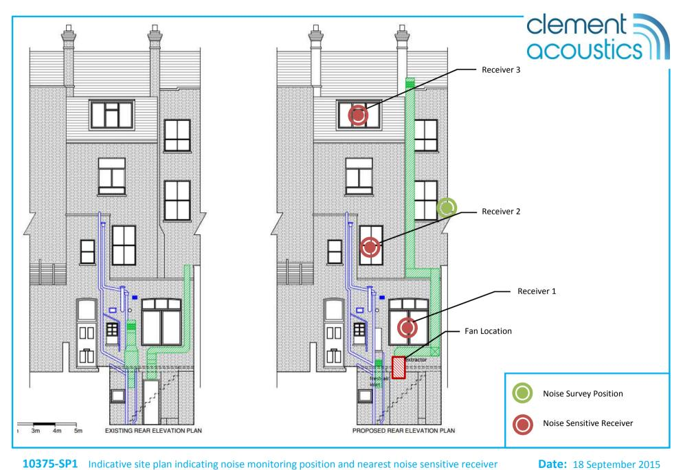
10375-SP1 Indicative site plan indicating noise monitoring position and nearest noise sensitive receiver
