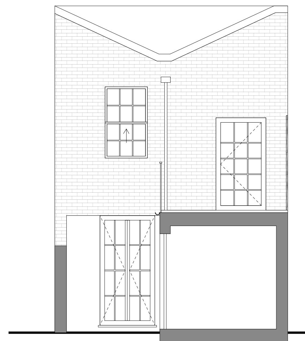
Rear Elevation Section
