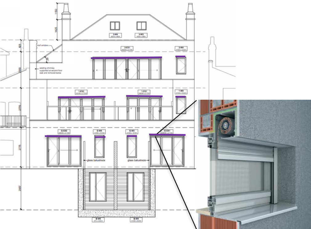
South facing windows with integral external blinds
