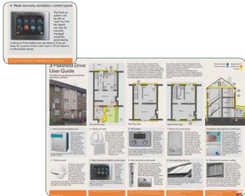
A simple home user guide will be produced to help the residents understand their new home and use it efficiently (e.g. MVHR controls)
