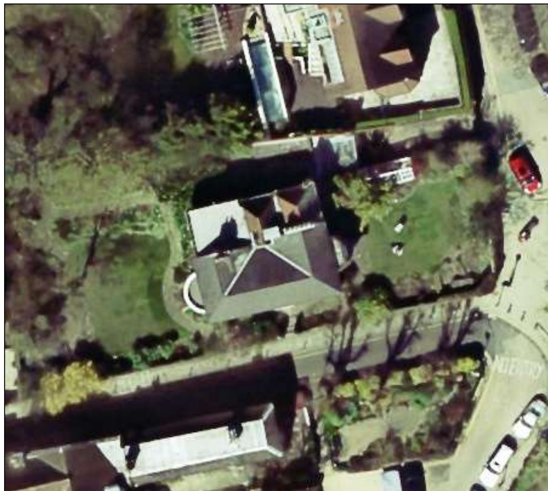
Plate 154 - Aerial photograph of current roof of Vine House showing loss of central gully and two pitches to the rear (Getmapping 2015)
