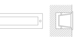
G50-300 Recessed wall luminaires with LED lamps in back of brick piers
