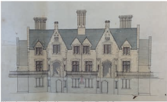
West elevation of school houses to Christ Church Passage
