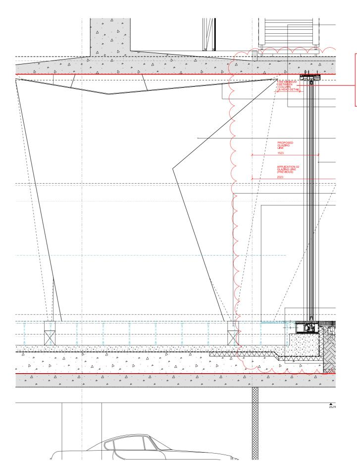
Note on drawing 552-15132 shows minimum **DIM** between glazing head detail for sliding door and column leading edge at 468mm
