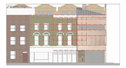
The proposed building is made up of horizontal bands and walls. Both are cast in situ and we suggest different surface treatments reflecting their different nature:
