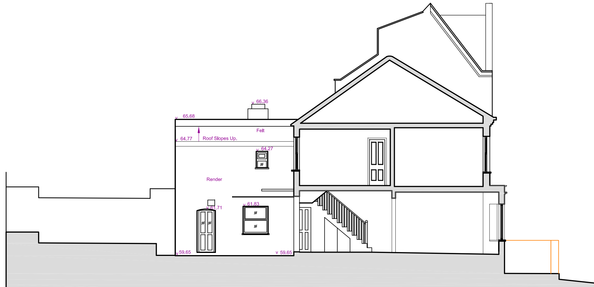
03. Side Return Elevation and Section (West Elevation)
