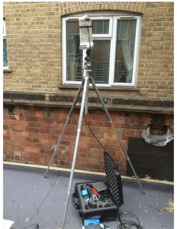
View of sound level meter measuring background noise near residents at rear, on flat roof.
