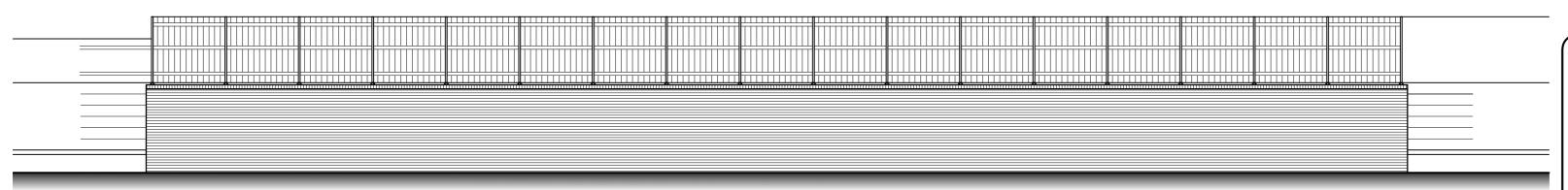
existing concrete plinth removed. New brick retaining wall constructed in front of existing PC Conc panel fence.
