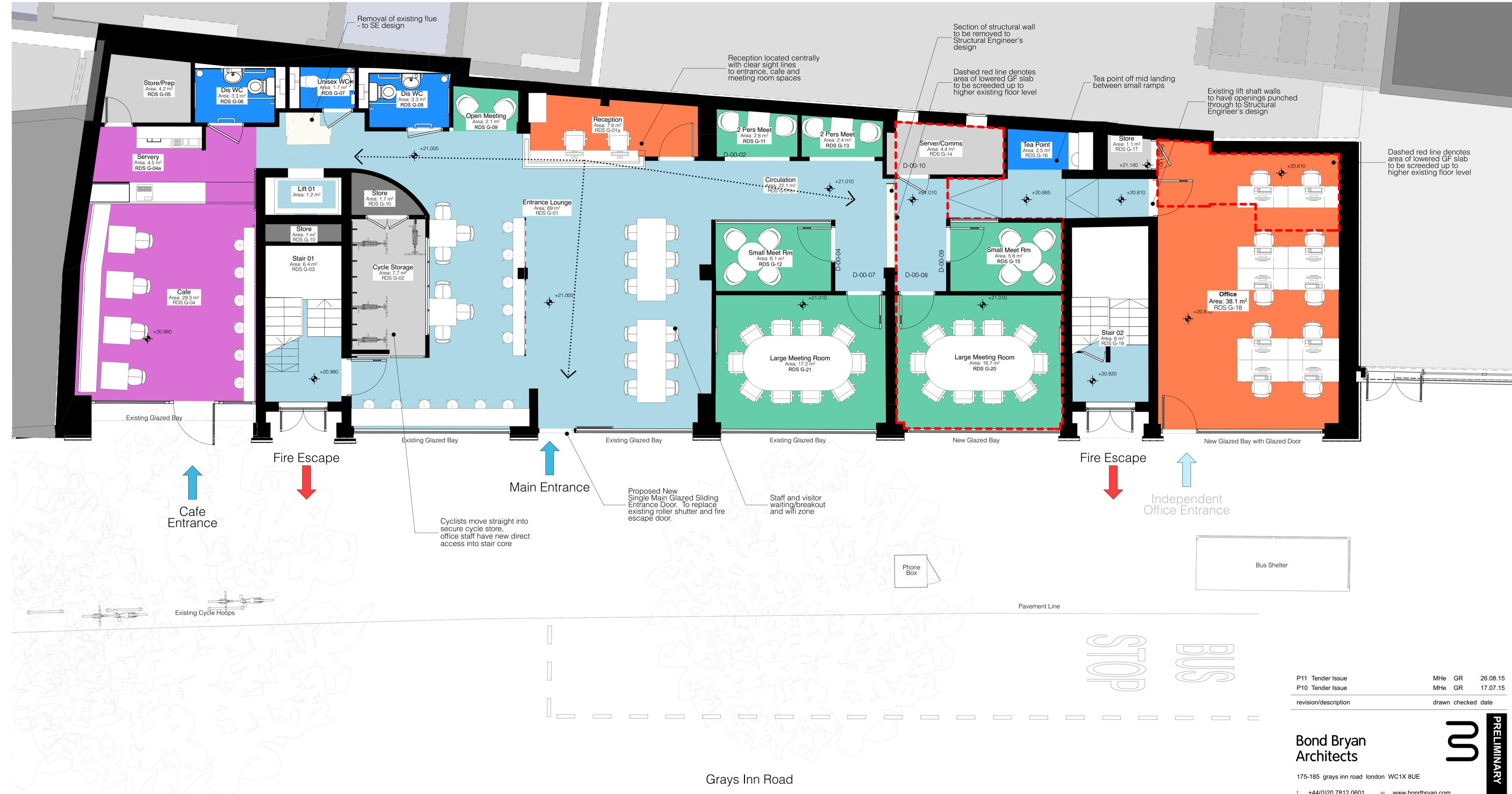
Survey information as per MT Surveys Data. Hatching indicates structure to be demolished - to SE design
