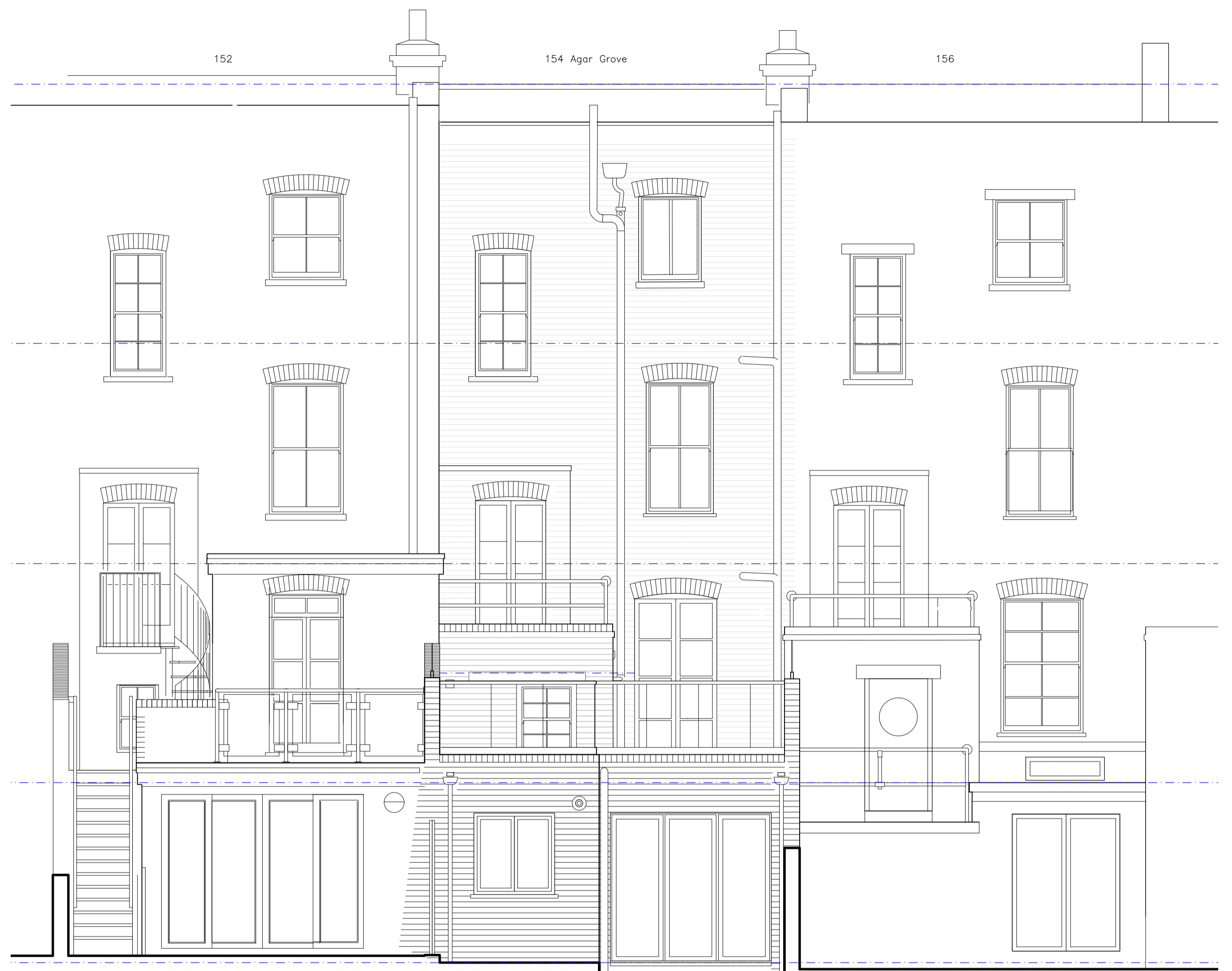
02 South Elevation PROPOSED & APPROVED 1:50 SHOWING APPROVED EXTENSION TO 152 AGAR GROVE PLANNING APPLICATION REFERENCE 2014/2428/P
