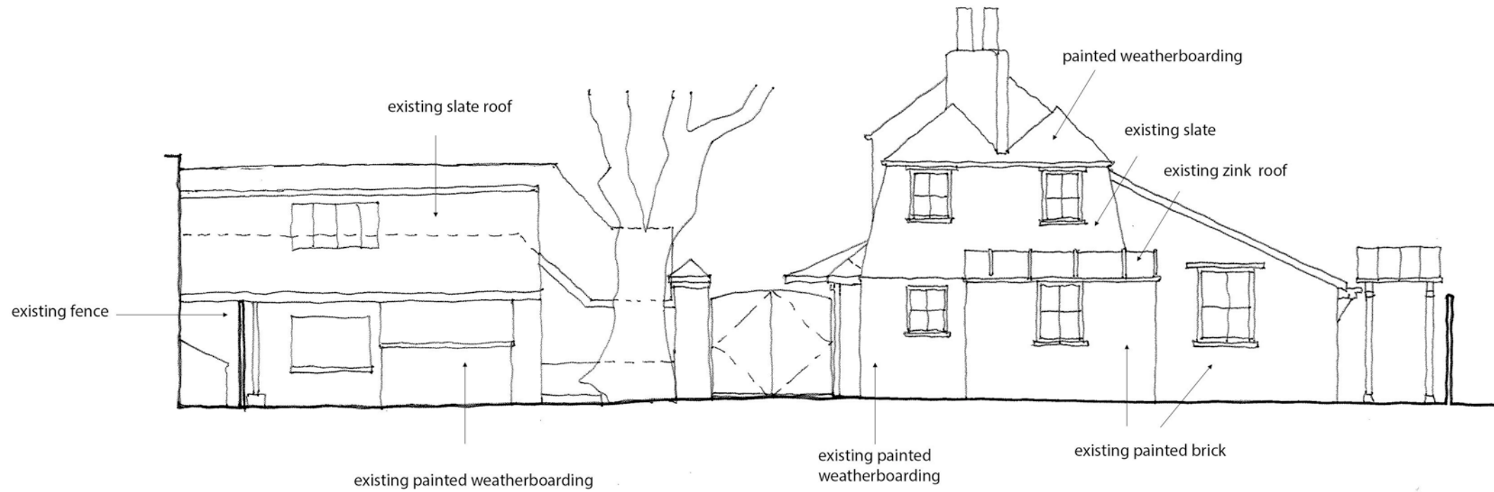
Existing East Elevation
