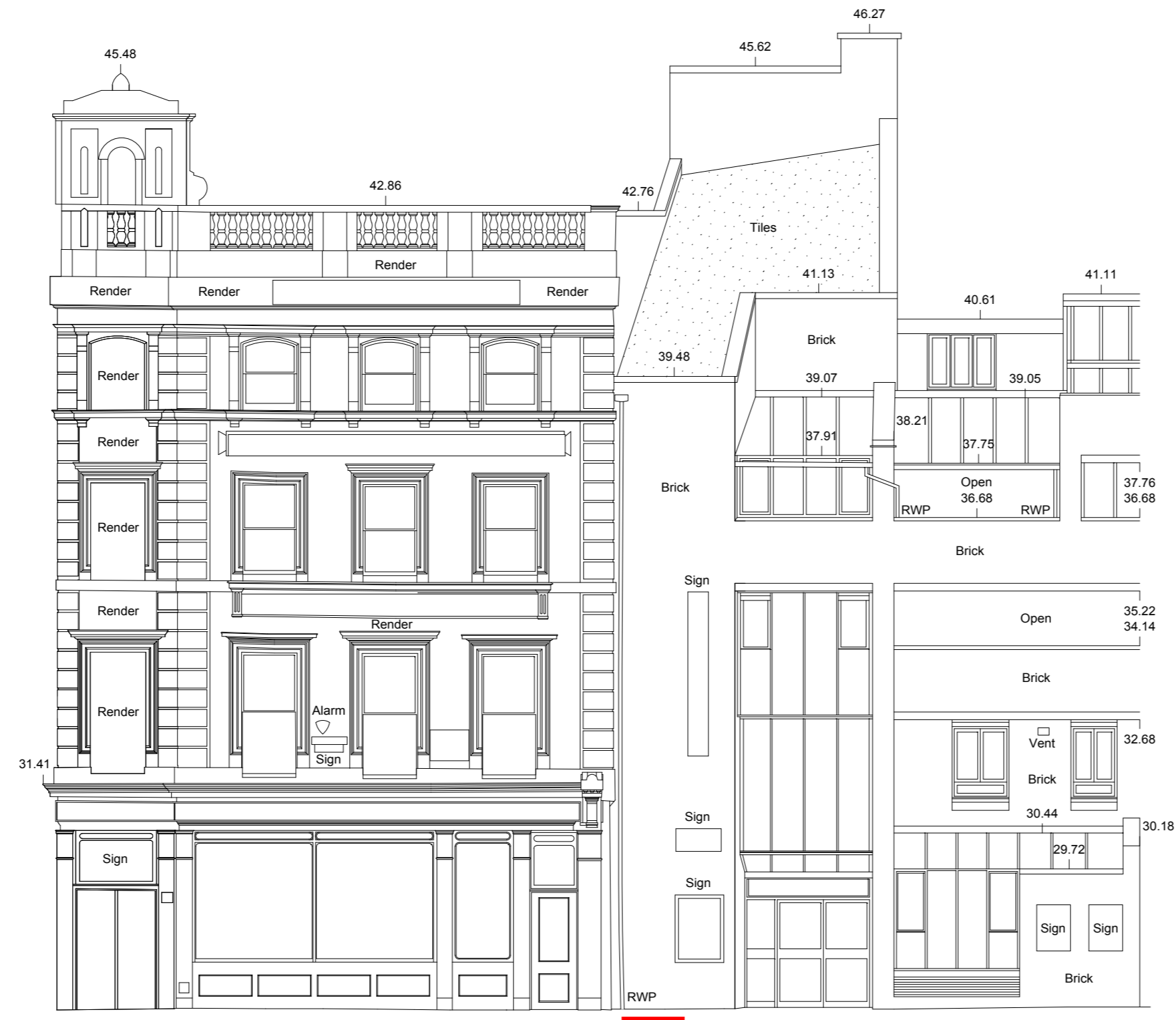
2 West Elevation (Hampstead Road) Scale: 1:100
