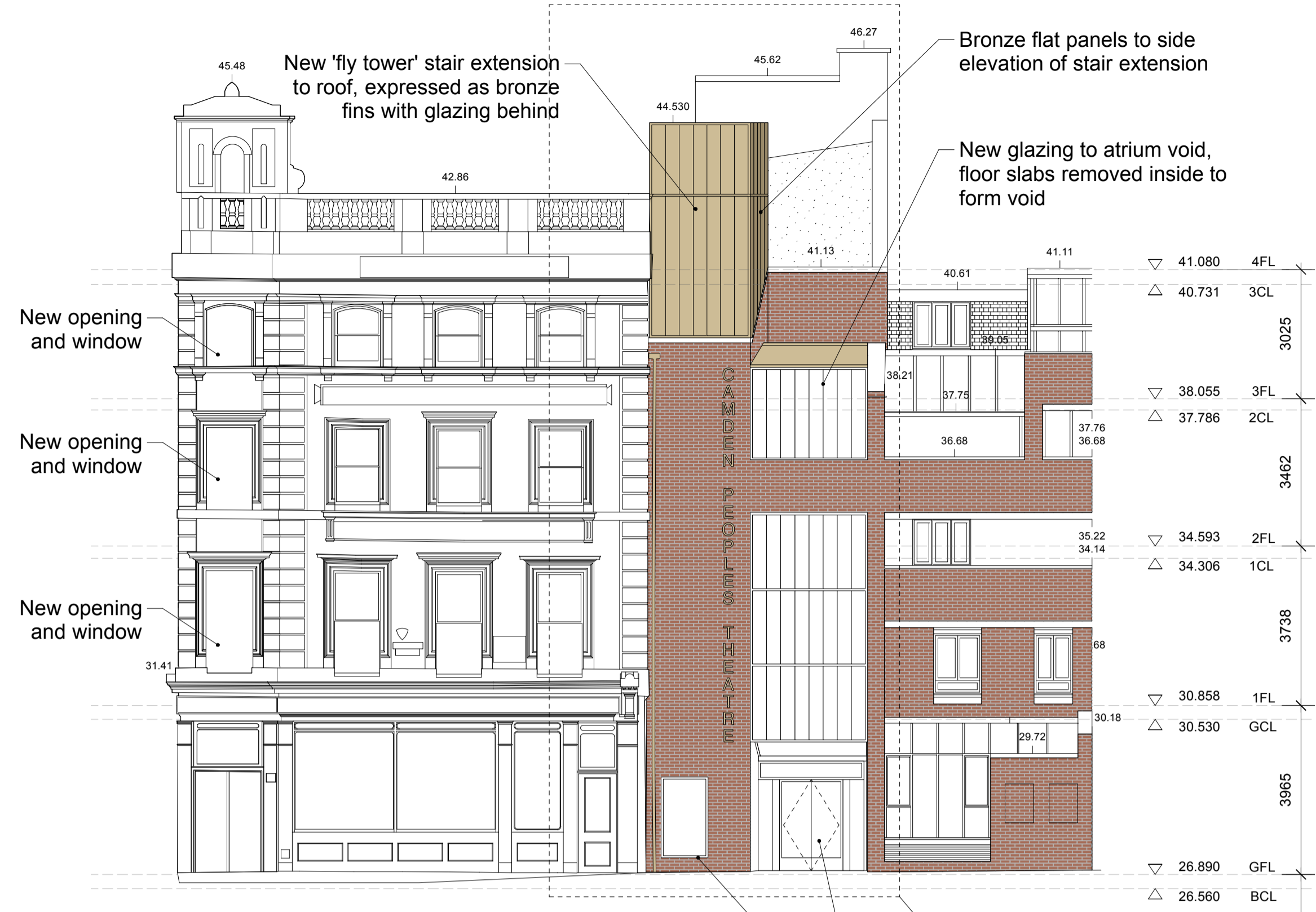
2 West Elevation (Hampstead Road) Scale: 1:100
