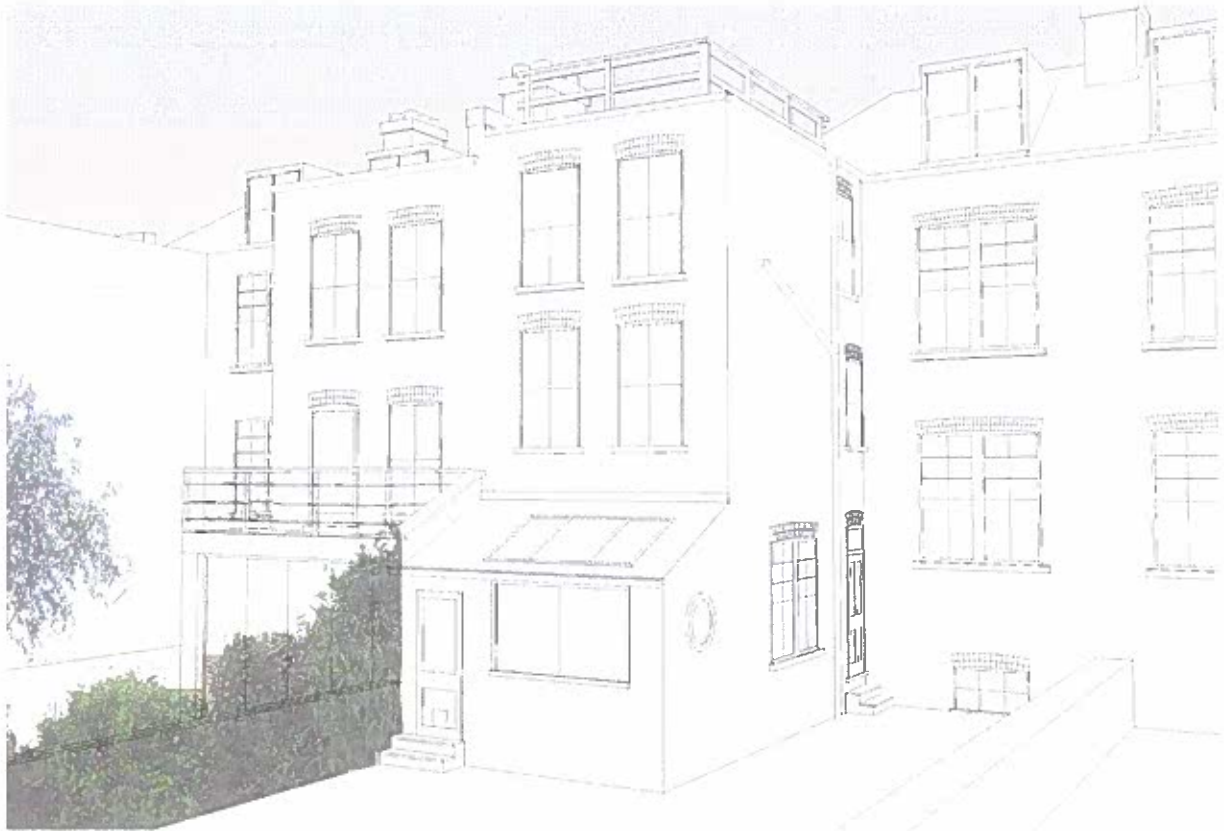
Existing rear elevation showing existing ground floor lean-to and third floor terrace balustrade
