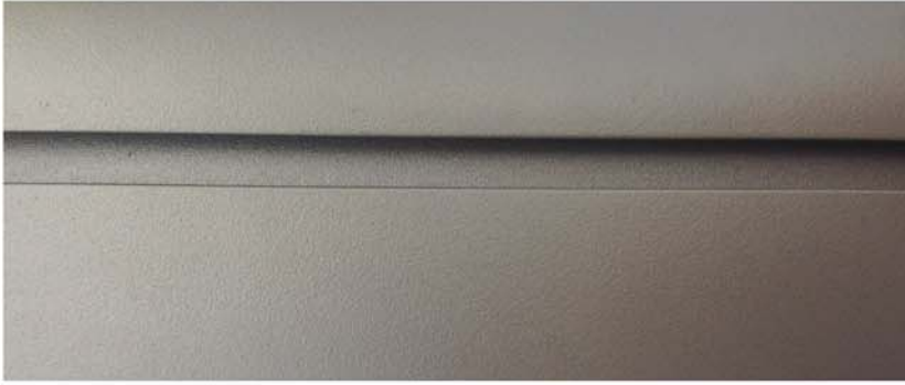
Metalwork: Entrance, window frames, pergola uprights. Powder coated aluminium/steel - Interpon - Gris: 2500 Sable: Futura
