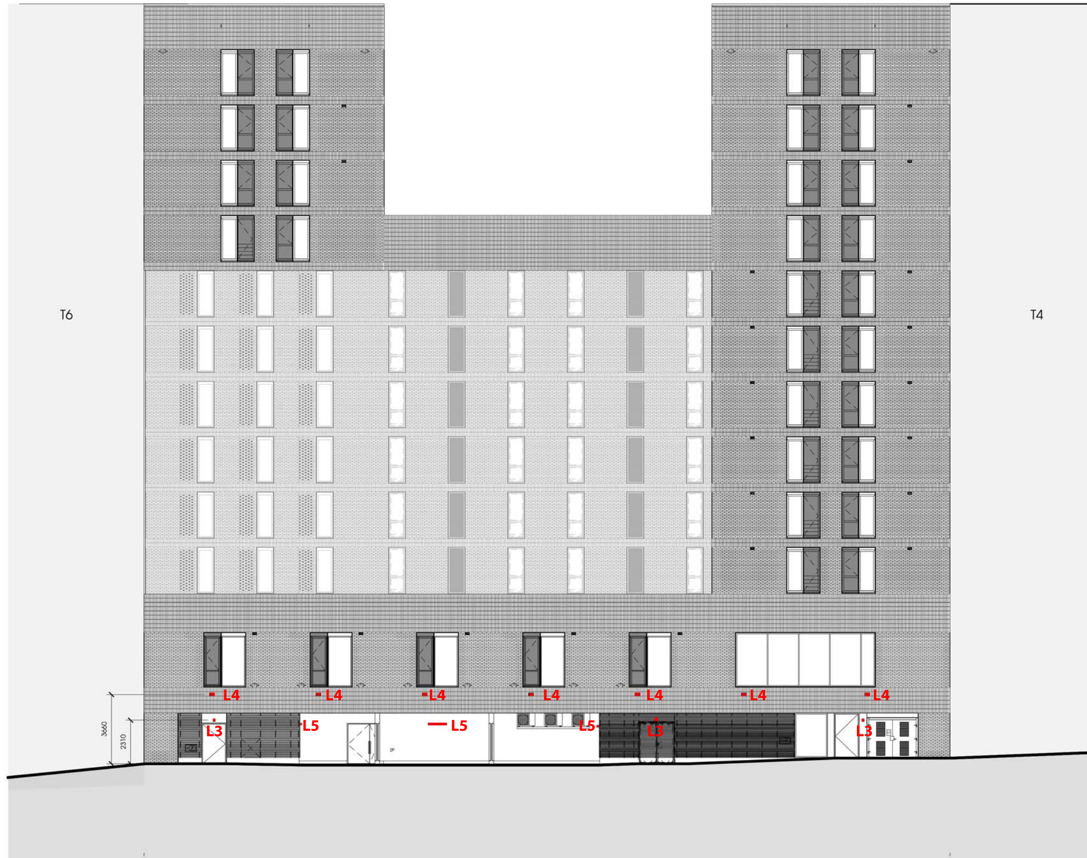
Building T5 SK_P7_North Elevation Lighting -See lighting data sheets for fitting types
