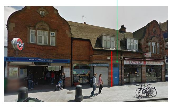
Vertical red line indicates route of new external gas pipe installed by National Grid. The gas pipe will enter the first floor flat just below the first floor window.
