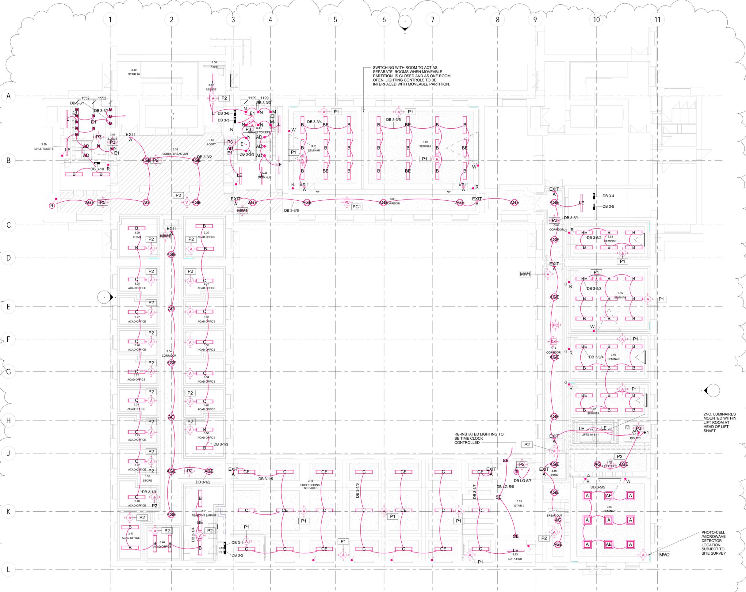
SWITCHING WITH ROOM TO ACT AS SEPARATE ROOMS WHEN MOVEABLE PARTITION IS CLOSED AND AS ONE ROOM OPEN. LIGHTING CONTROLS TO BE INTERFACED WITH MOVEABLE PARTITION.
