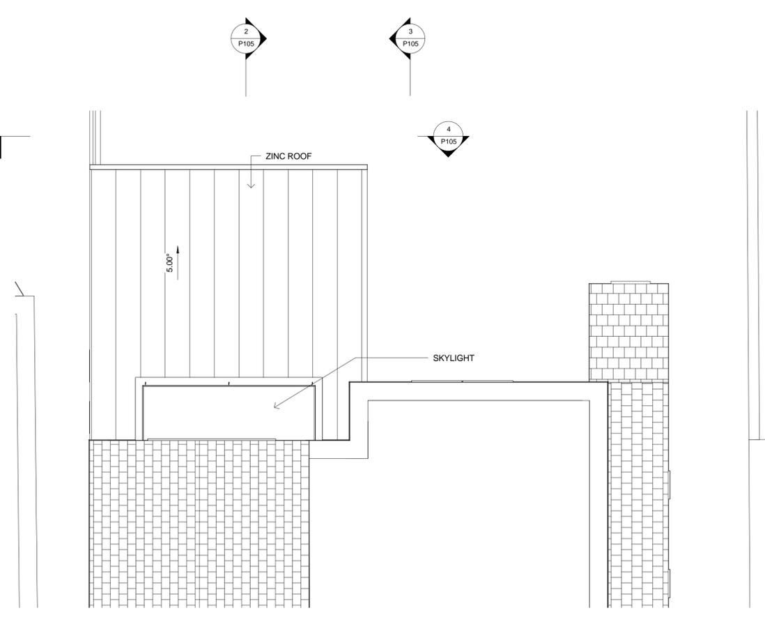
**3** PROPOSED FIRST FLOOR PLAN (EXTENSION ROOF)
