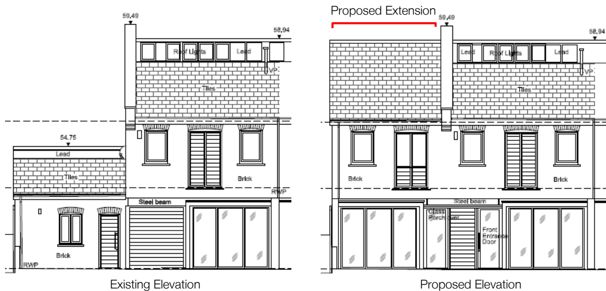
Figure 1-1 Existing and Proposed elevation of the scheme
