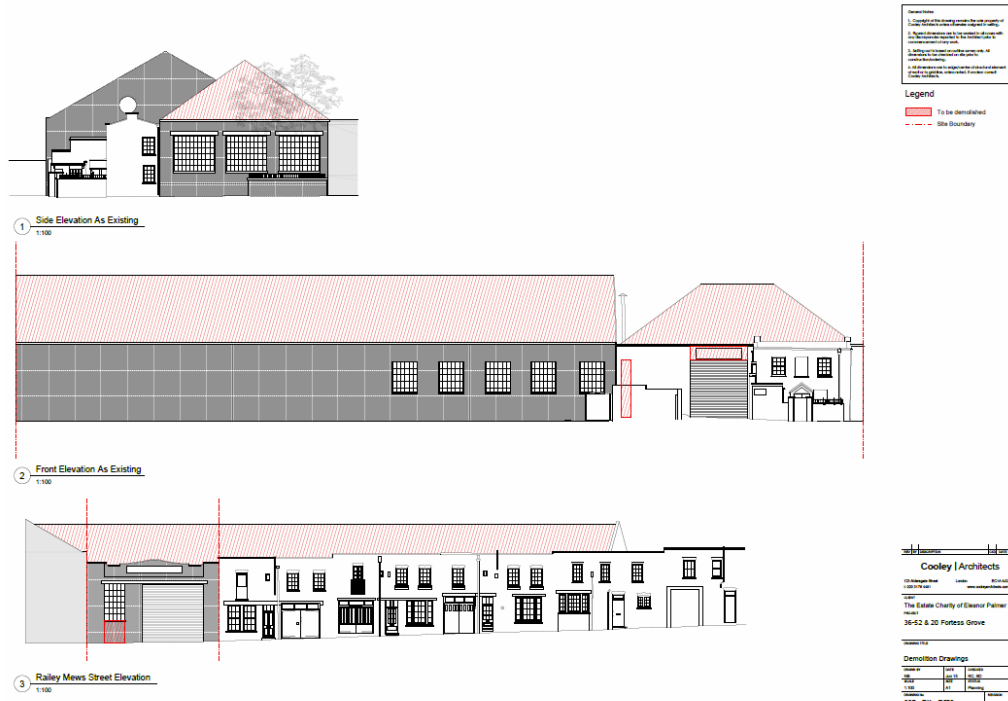
Figure 24: Demolition Drawings. Source: Cooley Architects (July 2015).
