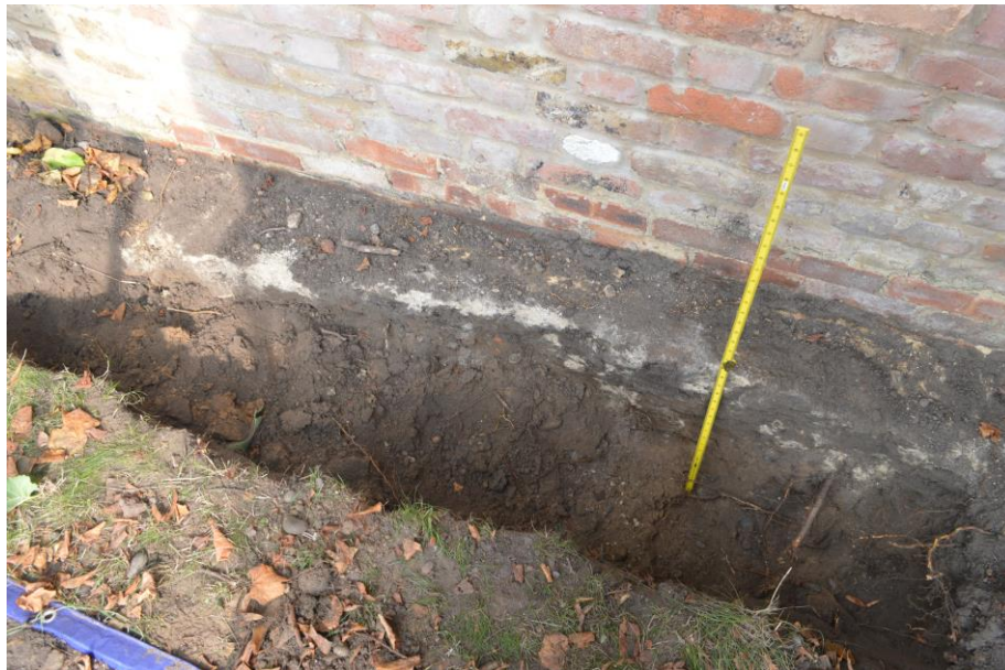
Photograph 2 Trench one showing no root activity from tree nos. 5 or 6.
