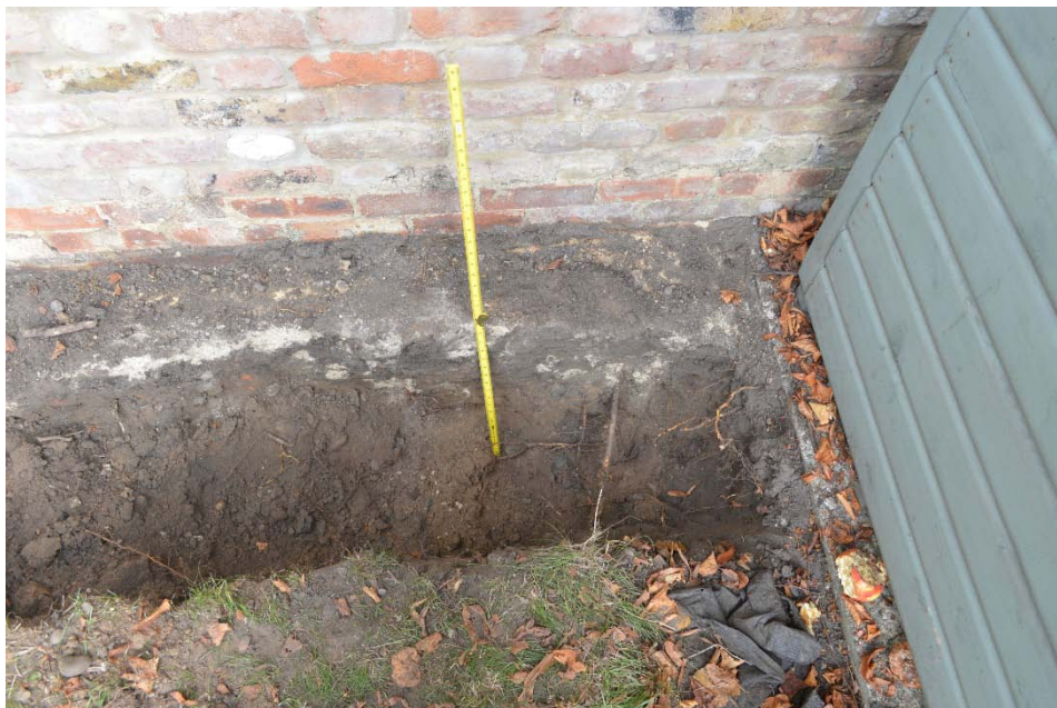
Photograph #3 – Showing the first stage of the excavation to a depth of 650mm with only one cypress root found
