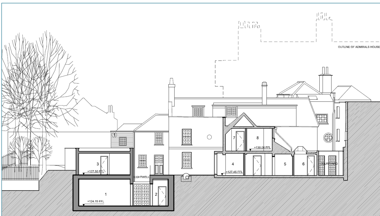
Figure 3.5: Proposed long-section through building and basement
