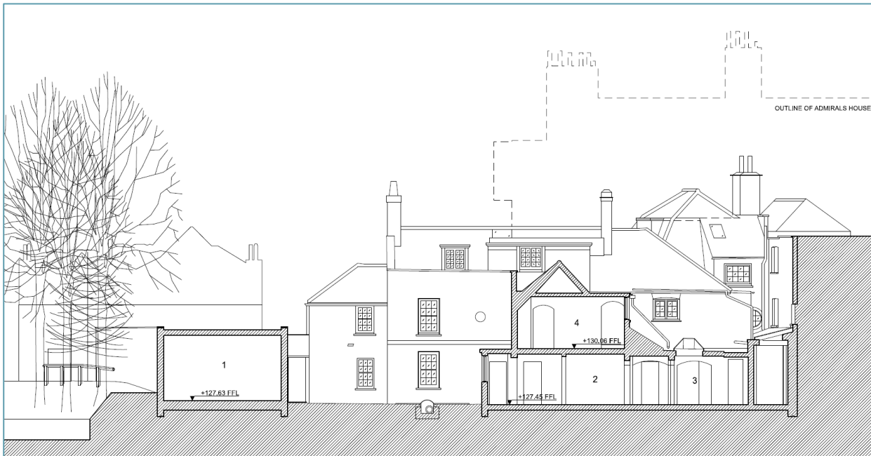
Figure 3.4: Existing building long-section
