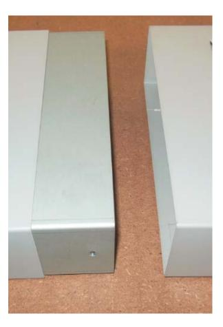
Typical coupling (generic metal work shown) – fittings will slide together and be secured via an internal stud. There will be no visible screws . Full manufacturing drawings will be provided when available.
