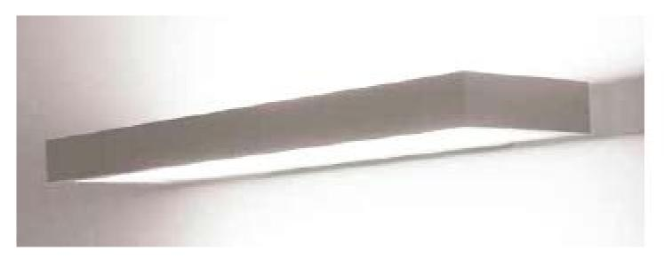
Reference: H1 Molto Luce System 01 570 – WL255E 2 x 55W fluorescent wall mounted up/downlighter fitting in RAL 9010 finish with dimmable gear. Manufactured from alluminium. 600mm W x 46mm H x 205mm D
