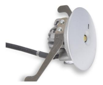
Reference: E Twintech Lighting Task 8020 3W non maintained recessed emergency downlight, in RAL 9010 Pure white finish aluminum housing, with narrow optic for corridor usage and 3 hour battery pack. 50mm dia. x 45mm H
