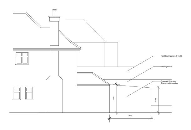
Proposed Rear and Side Elevation Drawing Number 02\_04 scale 1:100,@A4 Rev A
