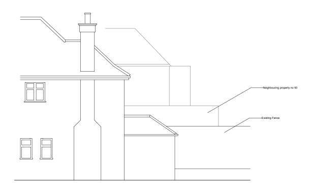
Existing Rear and Side Elevation Drawing Number 01\_04 scale 1:100,@A4 Rev A
