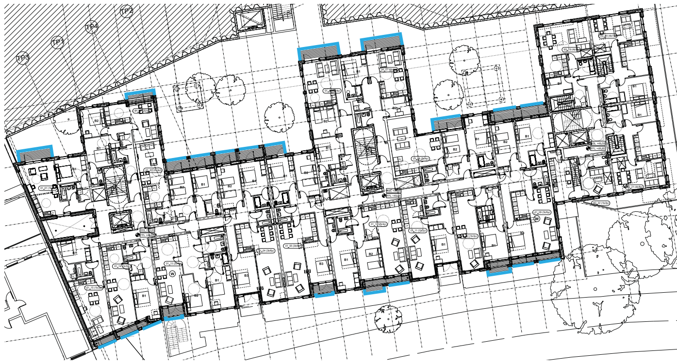
First Floor Typical locations of glazed balcony balustrading
