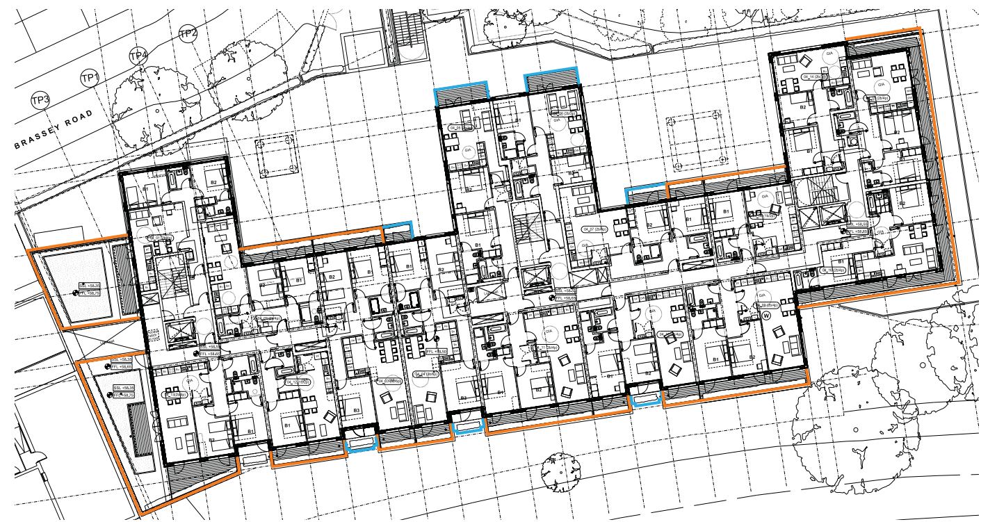
Penthouse Typical locations of glazed balcony balustrading Typical locations of terrace level brick parapet
