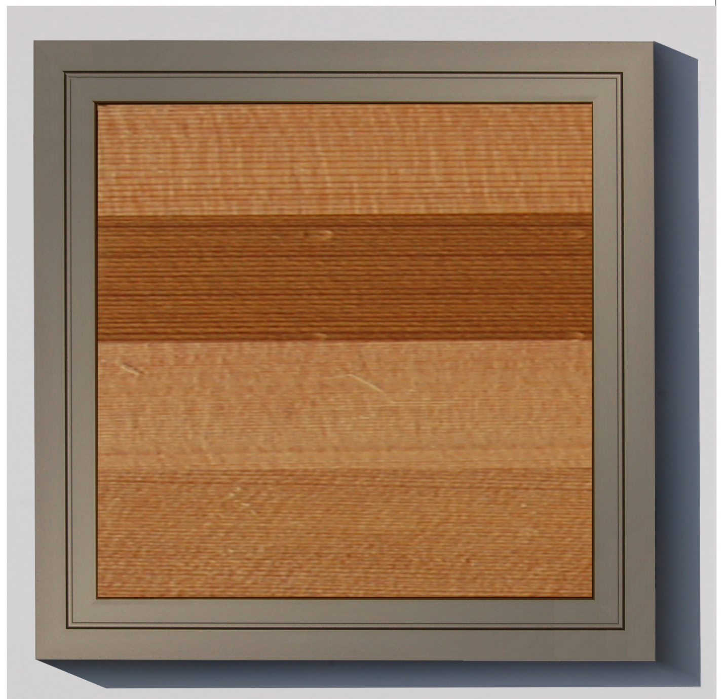
Proposed Western Red Cedar cladding material for solid panelling & light bronze finish for Velfac door & window frames
