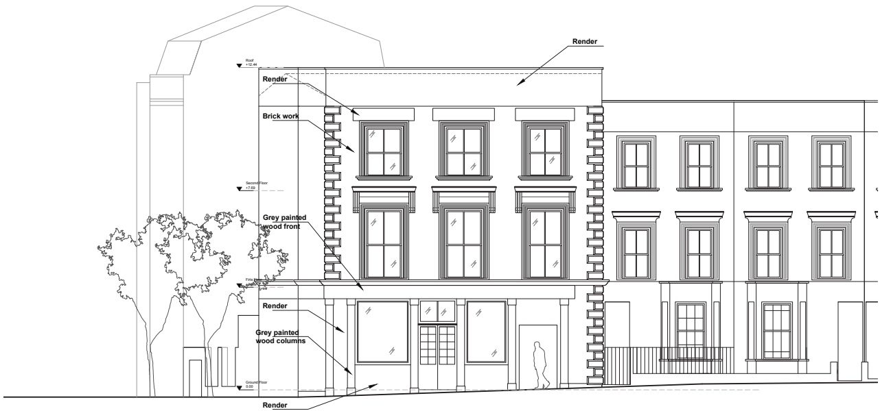
Existing elevation on Brecknock Road
