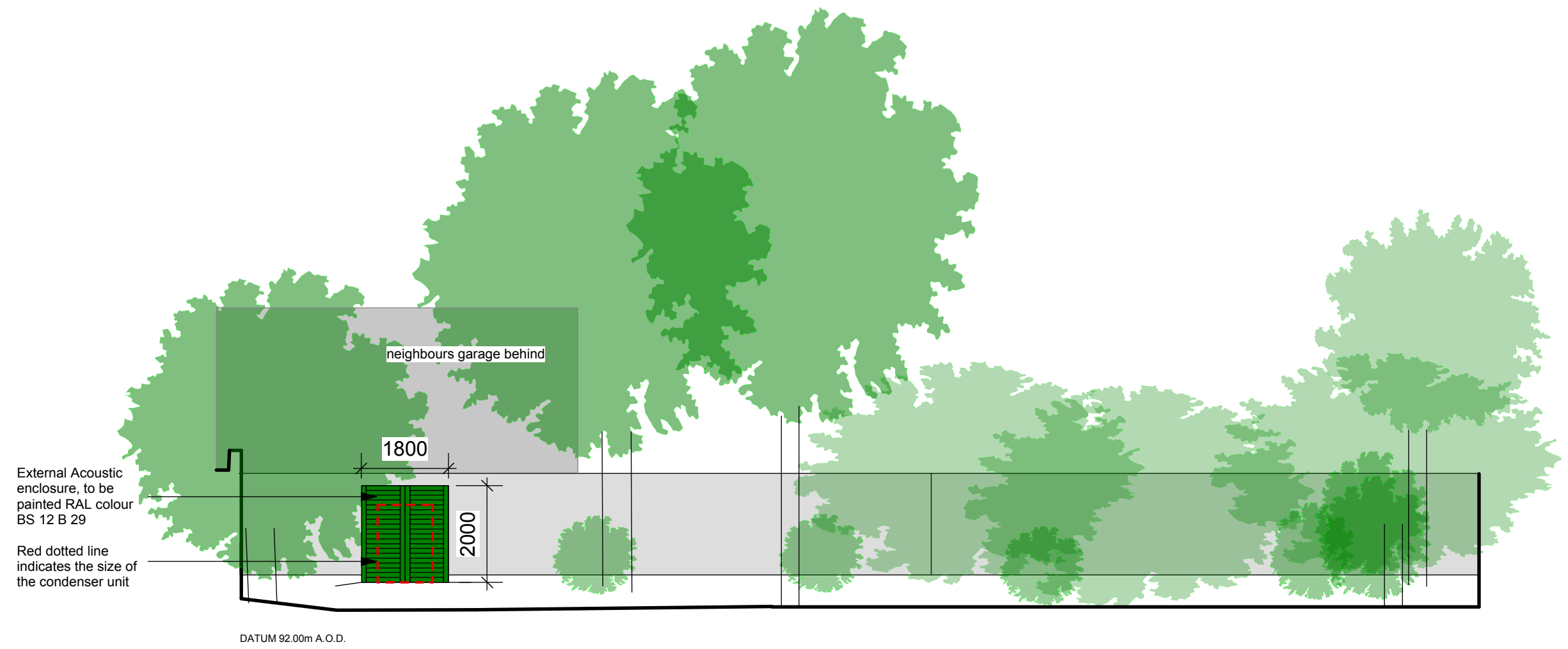
Condenser unit within External Acoustic Enclosure Scale 1:100
