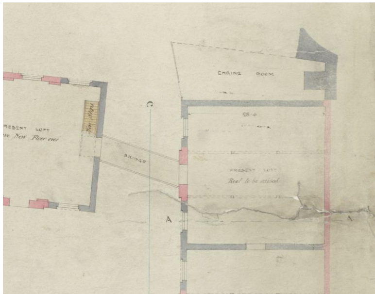
Figure 5 Close up of the 1880 plan of Tack Room showing the bridge connection between the Provender Store and the Tack Room
