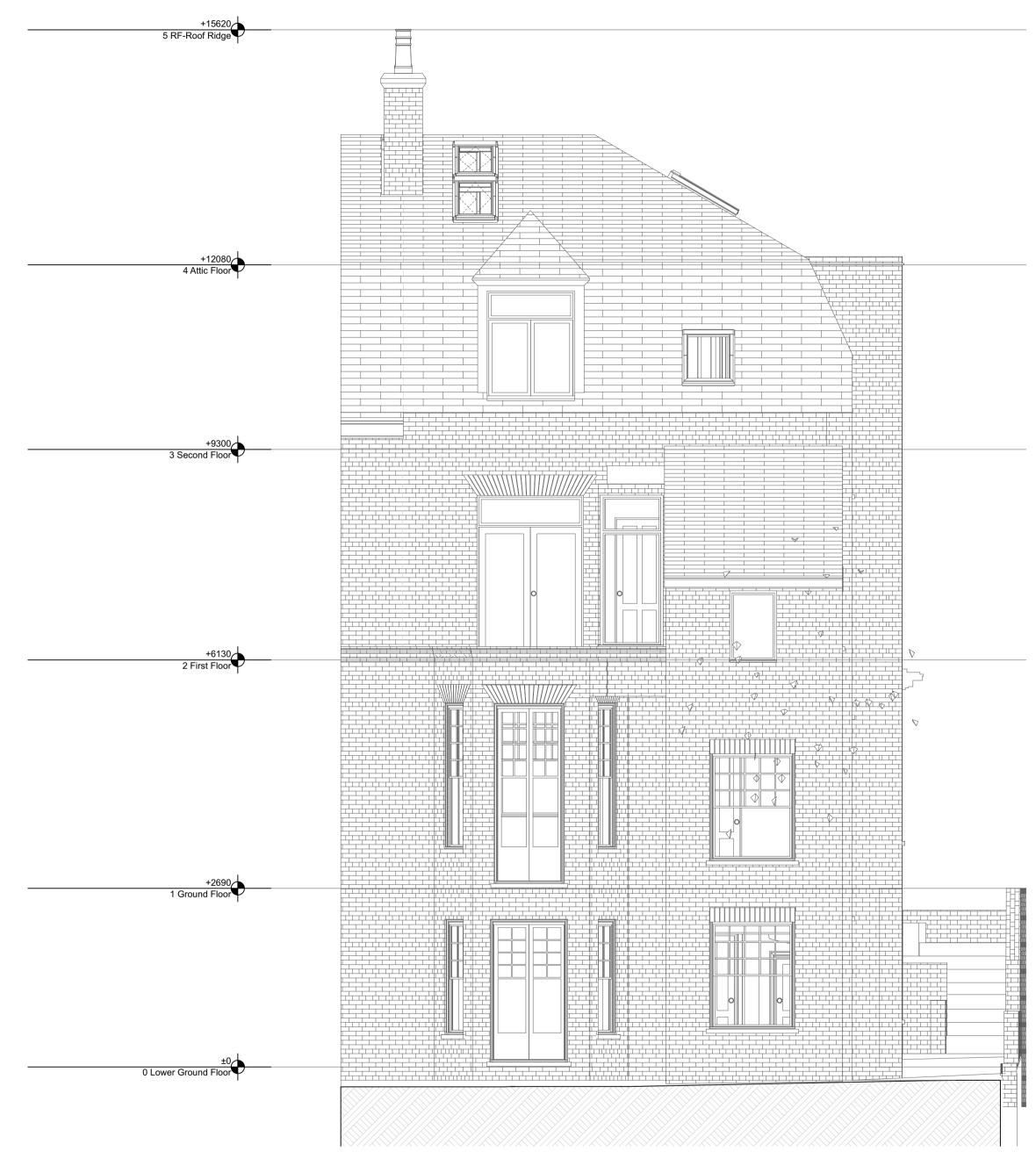
Section E-E / Rear Elevation as Existing 1:50
